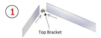
• Loosen set-screws in **TOP BRACKET** and slide a short and long piece of glass into it. (for square glass kits, all panels will be equally sized)
