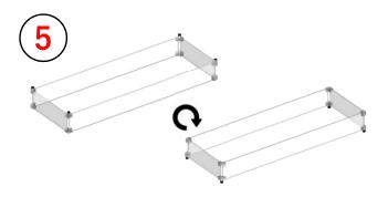
Carefully, using two people, flip the assembly over. Gently set the glass guard onto fire pit.
