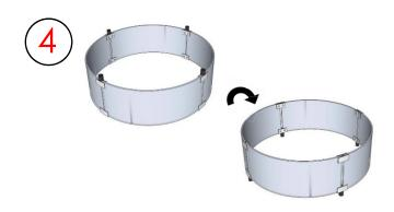
Carefully, using two people, flip fully assembled glass guard over and place on fire pit centered around burner.
